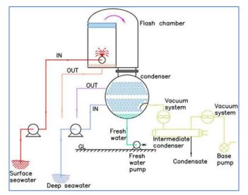
However, LTTD has its limitations, including the requirement for deep, cold water, which is not always available, and the relatively low production rate compared to other desalination technologies.
